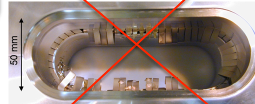
Damaged RF finger
