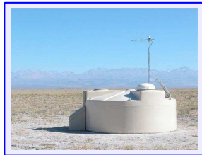
1600 Water-Cherenkov Detectors, \approx 3000 \text{ km}^2
