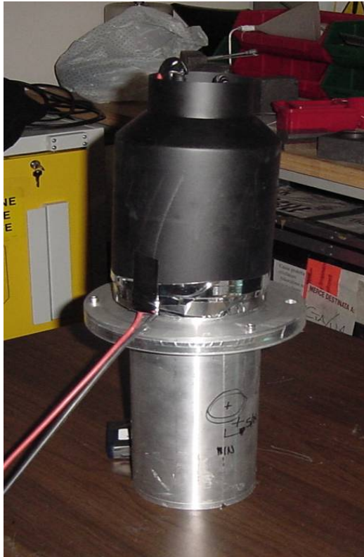
Re-cycled mu-metal shield (for testing purpose only)
