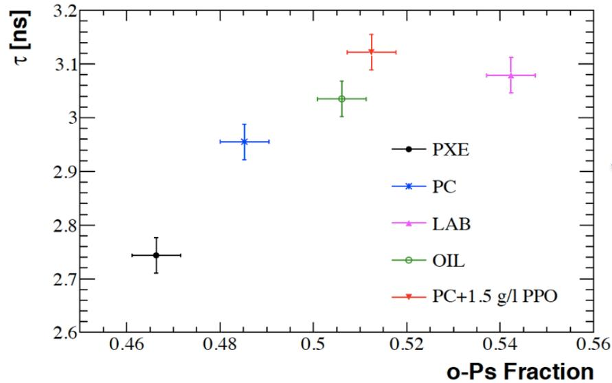
Measurements of the o-Ps meanlife and formation probability in scintillators with the PALS technique
