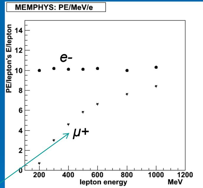
Number of detected photoelectrons per MeV as a function of lepton energy
