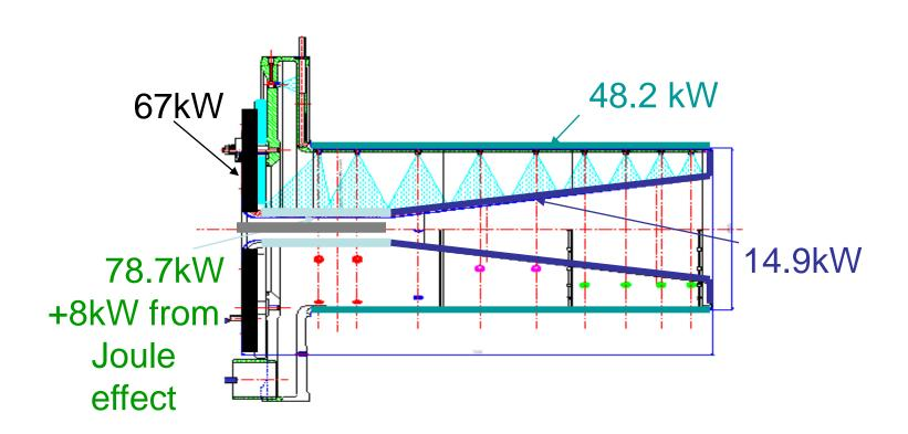
Total energy (particle + Joule)  $Q_{tot}150kW$ Increase of water tempearure  $\Delta T=15deg$ Water capacity at 20C  $c_p = 4183 \text{ J/kg/deg}$
