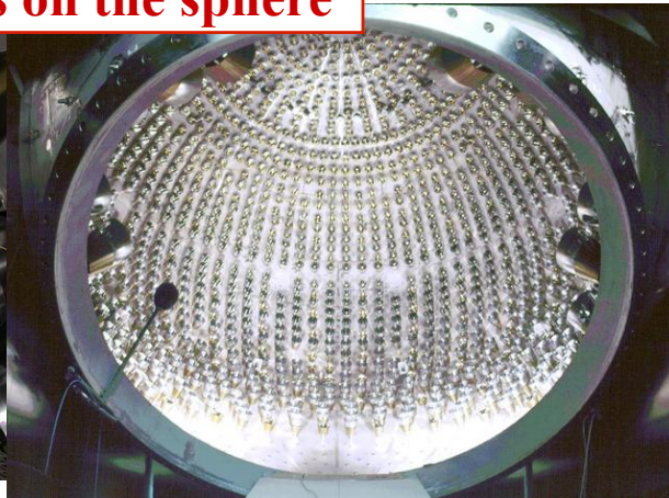
Installation of PMTs on the sphere
