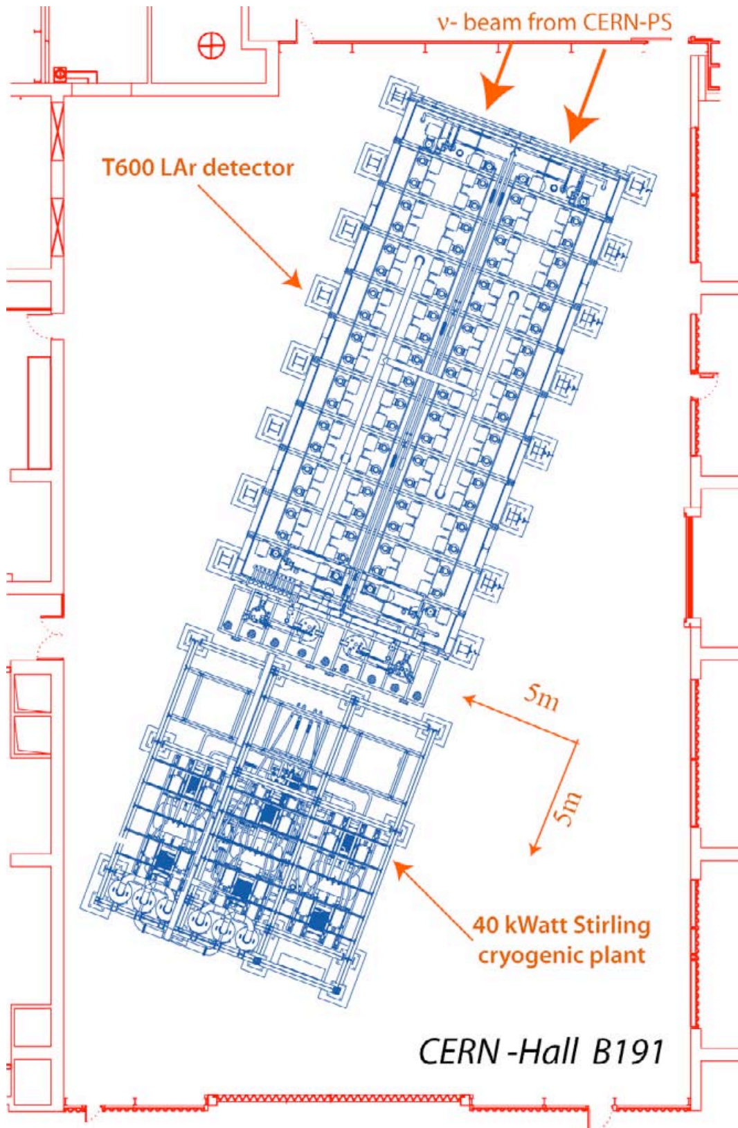
Figure 16. The general layout of the T600 LAr detector in the “Far” Position and of the associated cryogenic equipments in Hall B-191 at CERN. The direction of the neutrino beam is also indicated.
