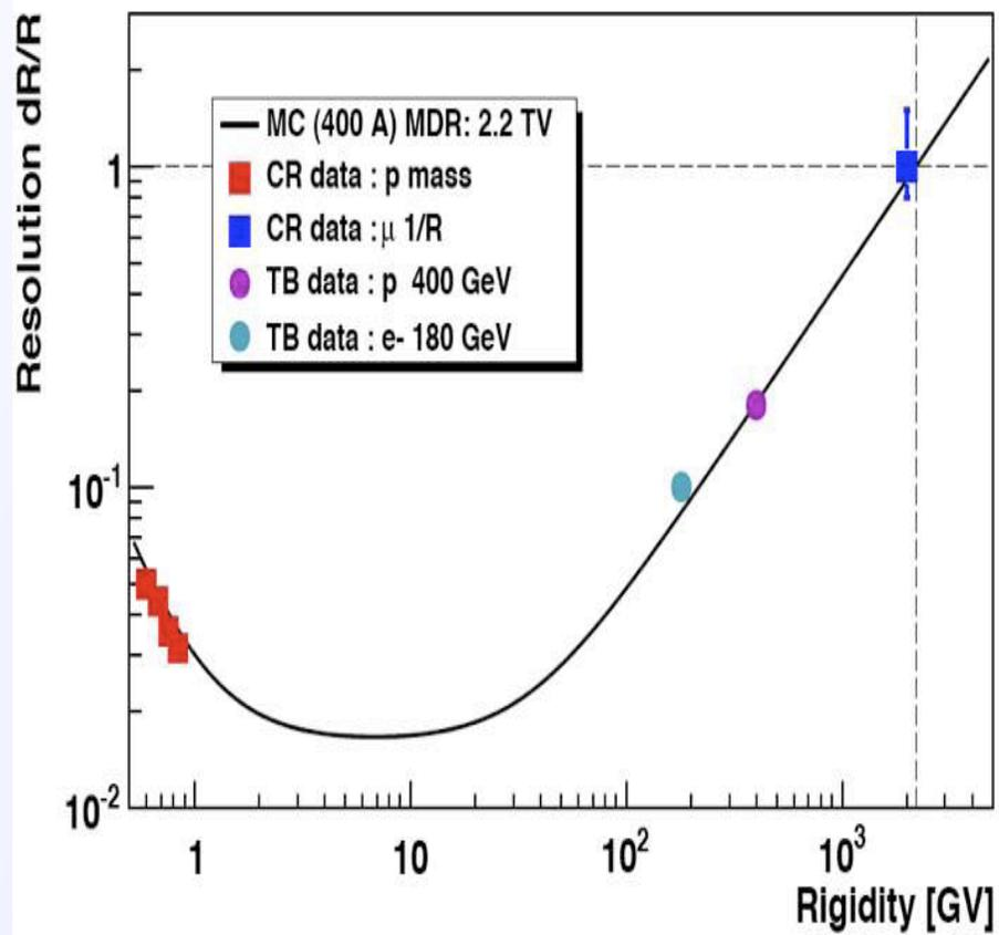
With 9 tracker planes, the resolution of AMS with the permanent magnet is equal (to 10%) to that the superconducting magnet.
