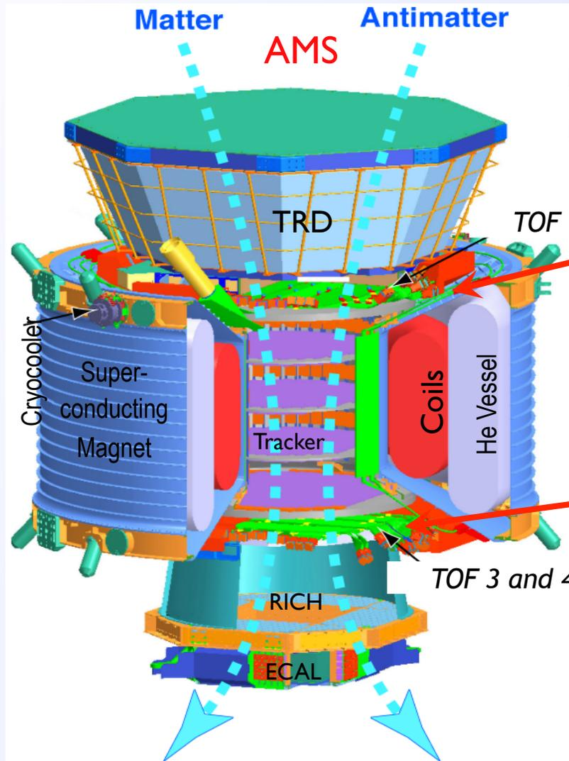
▷ Velocity measurement,  $v = \text{distance} / \Delta t$
