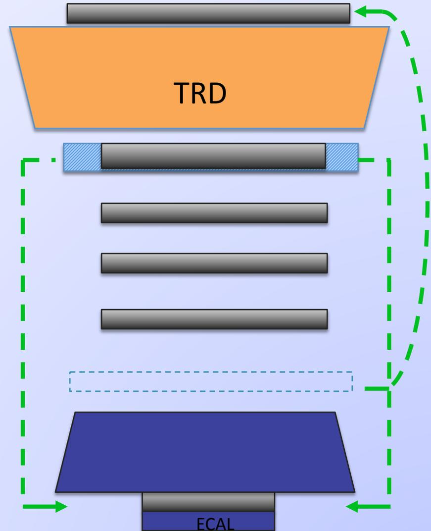
Layer 9 comes from moving the ladders at the edge of the acceptance from layer 1. The layer 8 is moved on top of the TRD to become IN. No new silicon and no new electronics .
