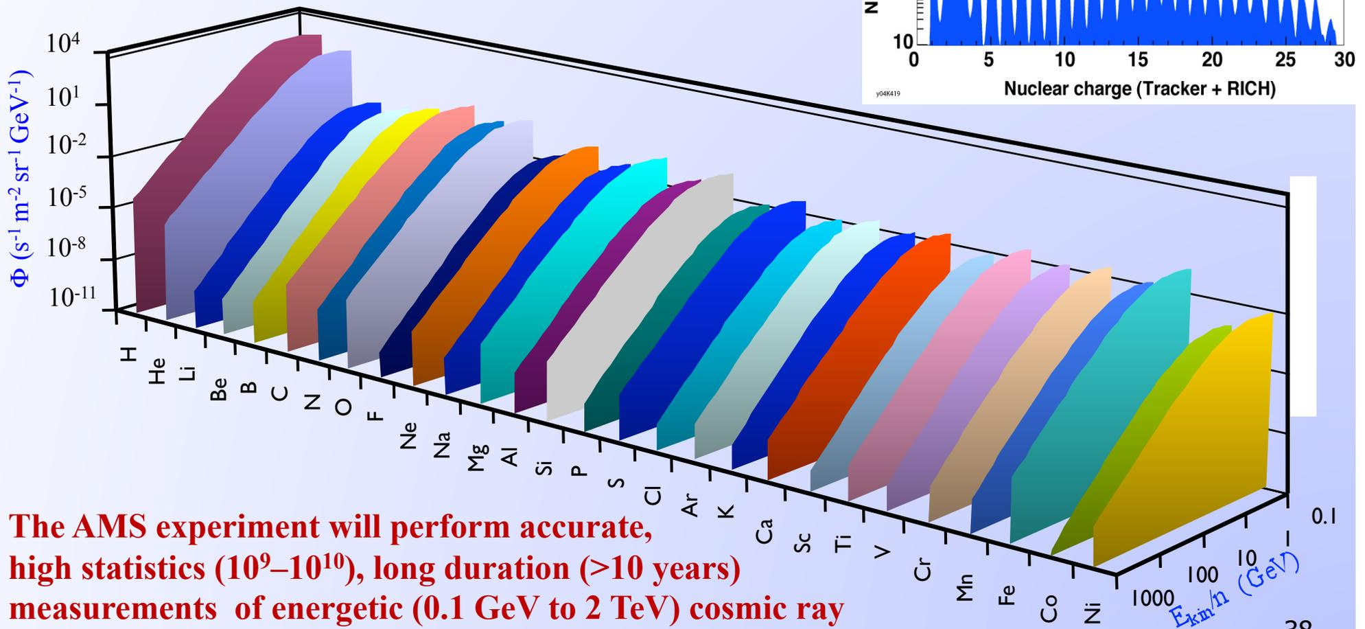
**The AMS experiment will perform accurate, high statistics ( $10^9$ – $10^{10}$ ), long duration (>10 years) measurements of energetic (0.1 GeV to 2 TeV) cosmic ray spectra in space.**
