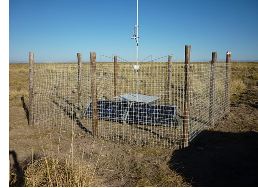
Self-Contained Radio Station (2008) 2 polar. f_{\text{middle}} \sim 65 \text{ MHz} Length = 3.22m Height = 1.40m 3KE/station
