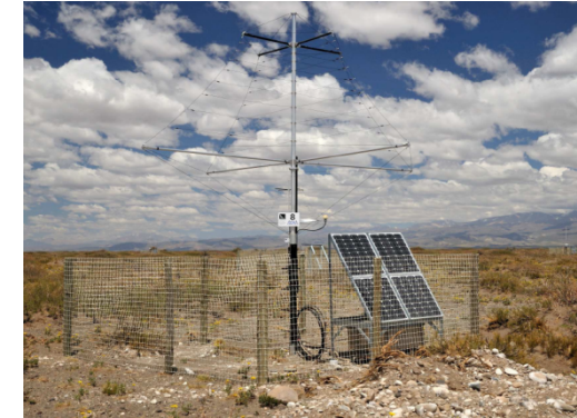
AERA Log periodic (2009) 2 polar. Diam = 6m Heigh = 6m Digital trigger
