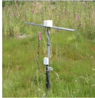
Active Short Fat Dipole (2006) length = 1.21m Height = 1m 50E/Antenna
