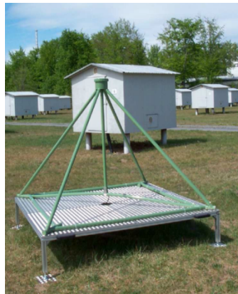
LOPES 2D (2005) V shape dip. 2 polar. Diameter = 2m Heigh = 1.5m
