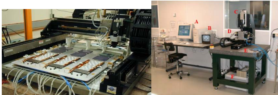
Fig.2. (Left) CMS gantry. A precision robotic assembly machine, where sensors are automatically aligned and glued. (Right) ATLAS assembly station.
