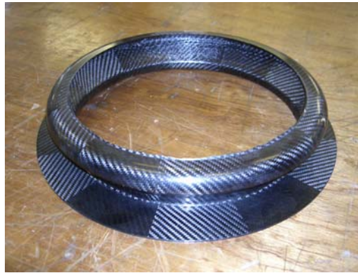
Figure 2 Part of the carbon fibre support frame for the MICE tracker which was designed and manufactured at the Oliver Lodge Laboratory in Liverpool.
