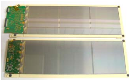
Photograph of the 2 modules with CMS sensors and 4VA1 & 1VA1+4SiTR_180ch. chips
