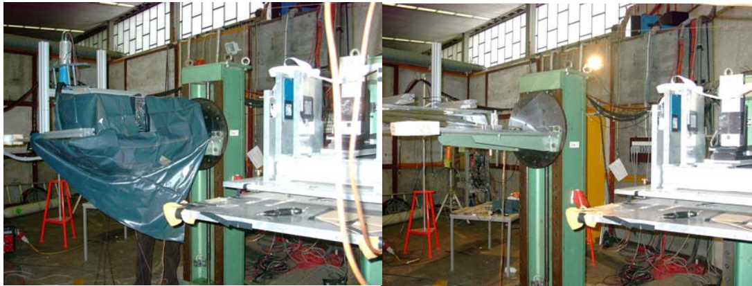
Photographs showing the test beam in DESY: on the left the 2 CMS modules installed in their Faraday box and similarly on the right the long ladder installed in its insulating box.
