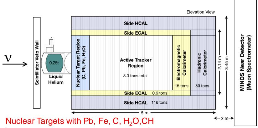
In same experiment reduces systematic errors between nuclei Side and downstream Calorimetry: Both Electomagnetic and Hadronic
