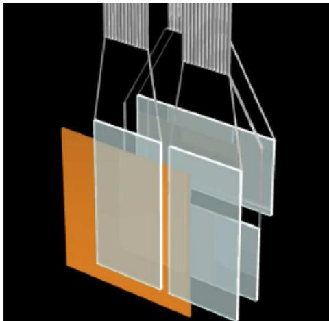
Front Counters: thin scintillators with  $8 \times 8\text{cm}^2$  acceptance installed in front of each main detector
