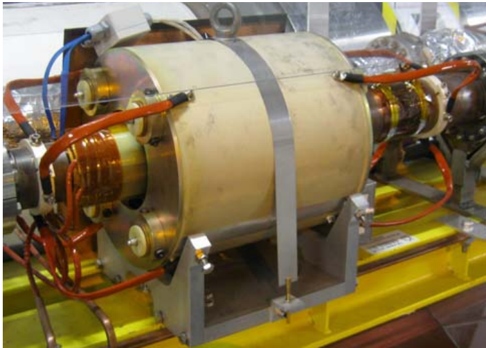
DCCT: DC Current Transformer Measures the total current
