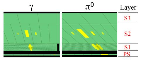
Fine granularity in S1 for  $\gamma/\pi^0$  separation
