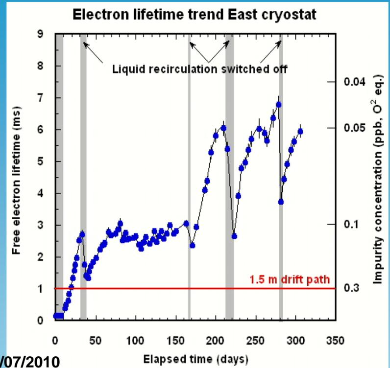
Simple model: uniform distribution of the impurities, including internal degassing, decreasing in time, constant external leak and liquid purification by recirculation.
