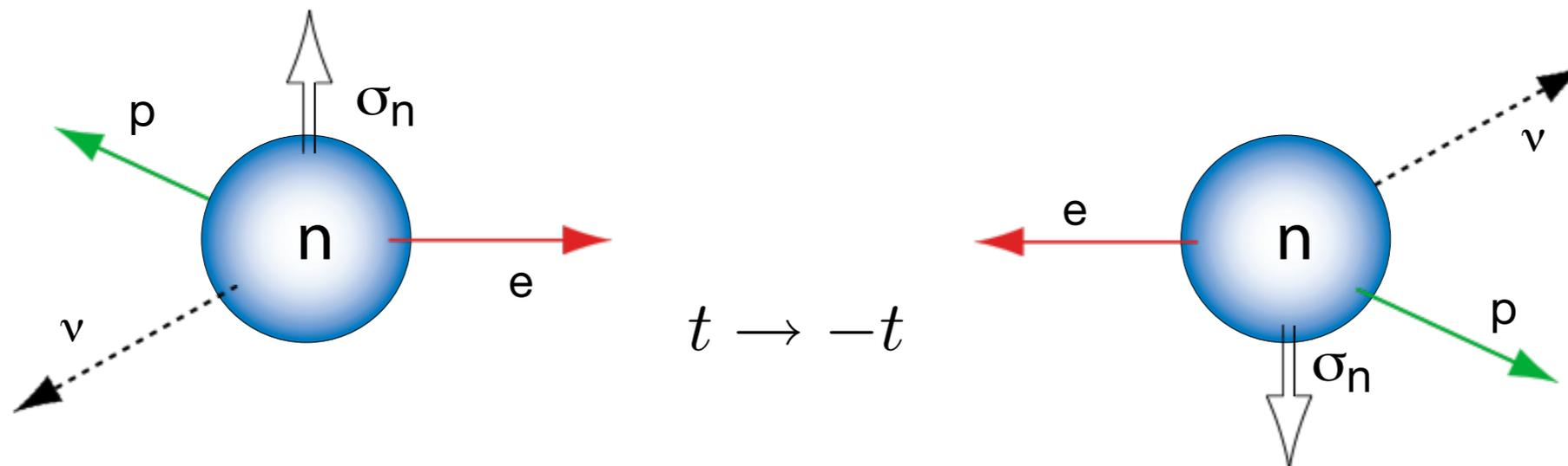
$$\frac{d\omega}{dE_e d\Omega_e d\Omega_\nu} = G(E_e) \left( 1 + \overset{\sim -0.1}{a} \frac{p_e \cdot p_\nu}{E_e E_\nu} + \sigma_n \cdot \left( \overset{\sim -0.1}{A} \frac{p_e}{E_e} + \overset{\sim 1.0}{B} \frac{p_\nu}{E_\nu} + \overset{\text{T-odd, P-even}}{D} \frac{p_e \times p_\nu}{E_e E_\nu} \right) \right)$$
