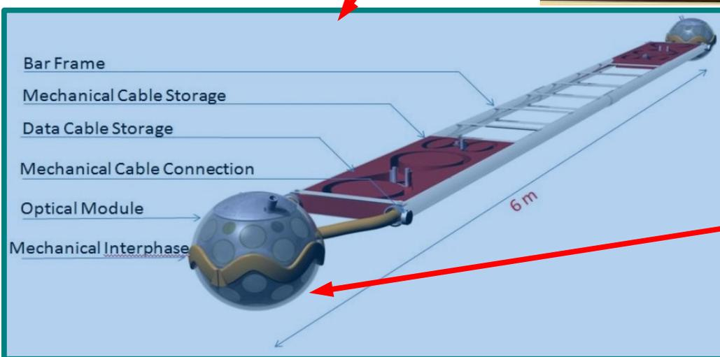
Detection Unit (DU): mechanical structure holding OMs, environmental sensors, electronics,...
