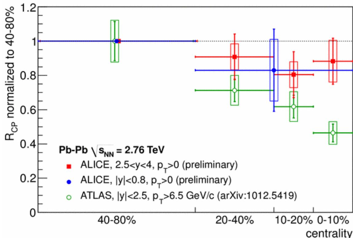
The  $R_{CP}$  extracted in ALICE at forward rapidity is not in agreement with the one extracted by ATLAS at mid-rapidity, especially in central collisions
