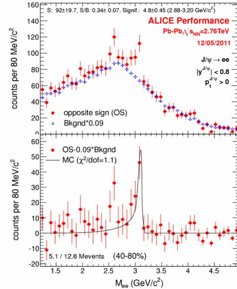
Data were taken at 2.76 TeV in both channels - total luminosity of  $2.7 \mu\text{b}^{-1}$
