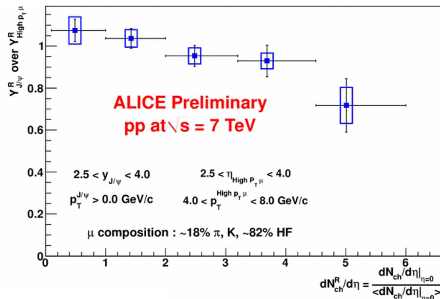
The J/ψ yield exhibits a weaker increase with  $dN_{ch}/d\eta$  than the high  $p_T$  muons (>80% of which are coming from heavy flavors). Different mechanisms can explain this observation such as kinematical effects, modification of the  $p_T$  distribution, modification of the bottom to charm ratio, etc..
