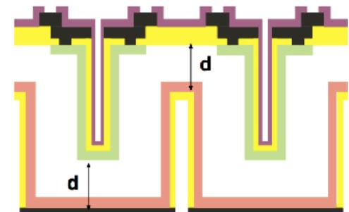
p+ etched and filled from bottom
