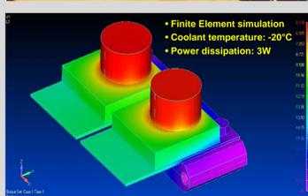
→ Measurements with infrared camera and FE calculations indicate  $\Delta T$  of ~ 15K to coolant temperature
