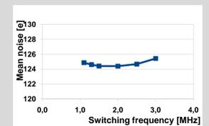
Noise of CMS pixel modules measured with and without DC-DC converter
