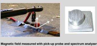
→ Shielding with 90µm thick Aluminium cap is sufficient
