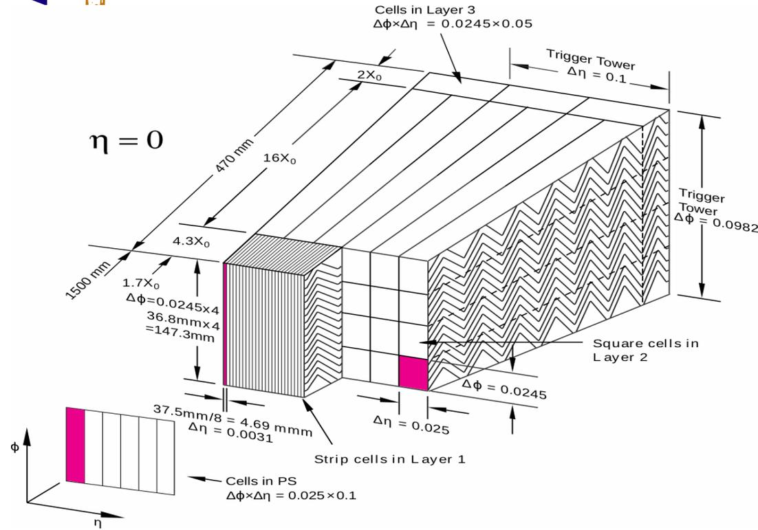
Calorimeter **granularity** crucial for reconstructing the **transverse energy shower profile** of hadronic tau decays and jets
