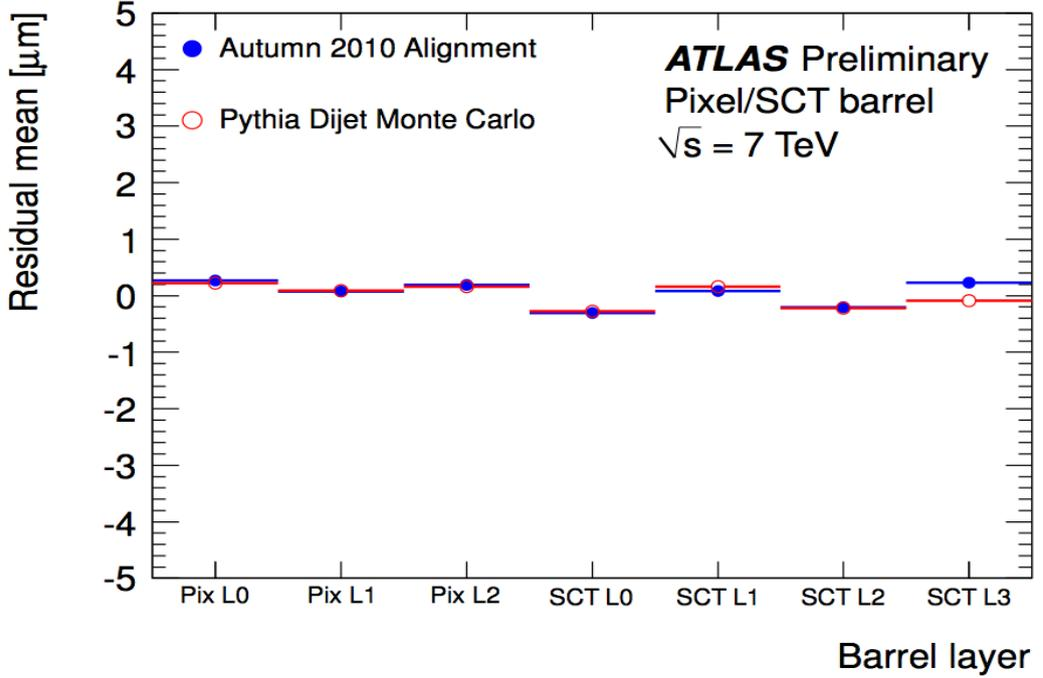
Good resolutions are necessary for precision tracking and secondary vertexing for tau candidates
