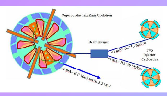
Use  $H_2^+$  and stripping extraction  $H_2^+$  binding energy 2.75 eV >> H<sup>-</sup> which is only 0.75 eV, so much more stable and easier to handle
