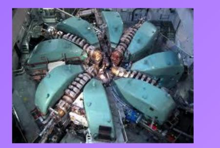
Isochronous Proton Synchrotron at PSI 590 MeV, 2.6 mA Well understood and very successful machine Not quite powerful enough – but not far off
