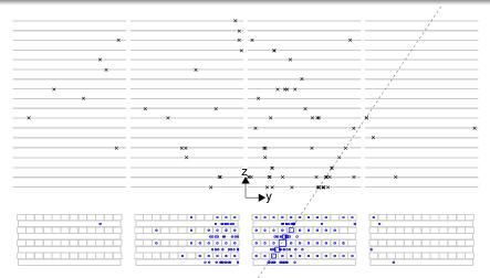
Angular resolution determined by hit resolution and lever arm
