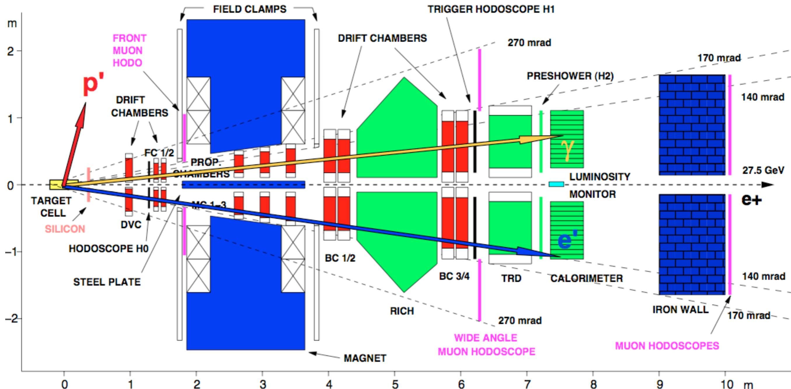
★ Measured photon and electron in forward spectrometer.
