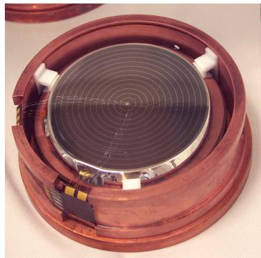
*EDELWEISS-II: WIMP search results with cryogenic germanium detectors with interleaved electrodes (ID)*
