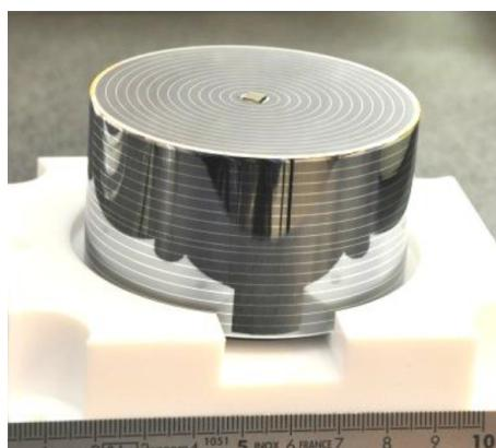
*EDELWEISS-III: large detectors fully covered with interleaved electrodes (FID)*
