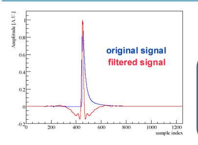
Data are divided in slices and then filtered in the frequency domain using the optimum filter algorithm, maximizing the signal to noise ratio
