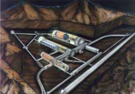
Laboratori Nazionali del Gran Sasso – **LNGS a natural shield** of 1500 m of rock (3650 meters of water equivalent. Average depht)
