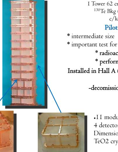
I Tower 62 crystals M ≈ II kg of <sup>130</sup>Te Bkg @ Q-vallue 0.17 c/keV/kg/yr Pilot experiment \* intermediate size ββ0υ experiment \* important test for \* radioactivity \* performance of large LTD arrays Installed in Hall A @ LNGS since middle of 2003 -decomissioned in June 2008-
