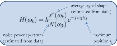
The trigger is implemented as a simple threshold trigger on the filtered samples, with debounce time related to the width of the filtered average pulse
