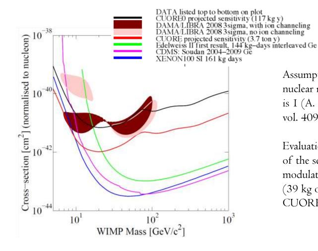
Assumption: quenching factor for nuclear recoils in TeO2 bolometers is I (A. Alessandrello et al., NIM A, vol. 409, pp. 451–453,1998).
