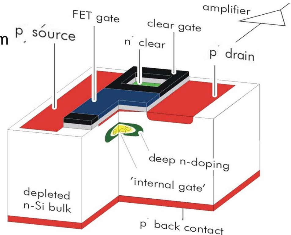
Fully depleted: → large signal, fast signal collection
