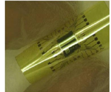
Fully functional microprocessor chip in flexib plastic envelope. Courtesy of Piet De Moo
