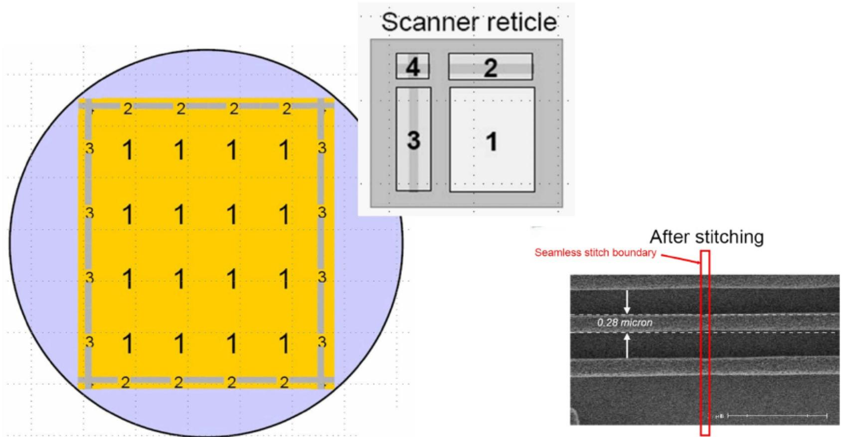
**Maximum length of monolithic ladder (8" wafer): 10 –15 cm**
