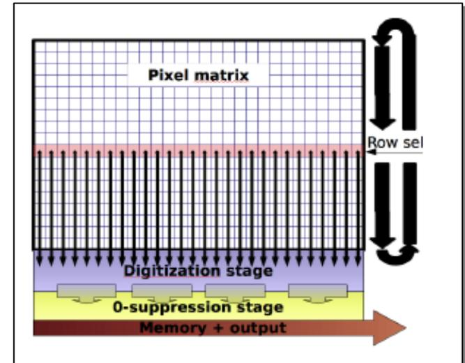
Priority given to high granularity, low material budget, low power consumption, with sufficient read-out speed and radiation tolerance.
