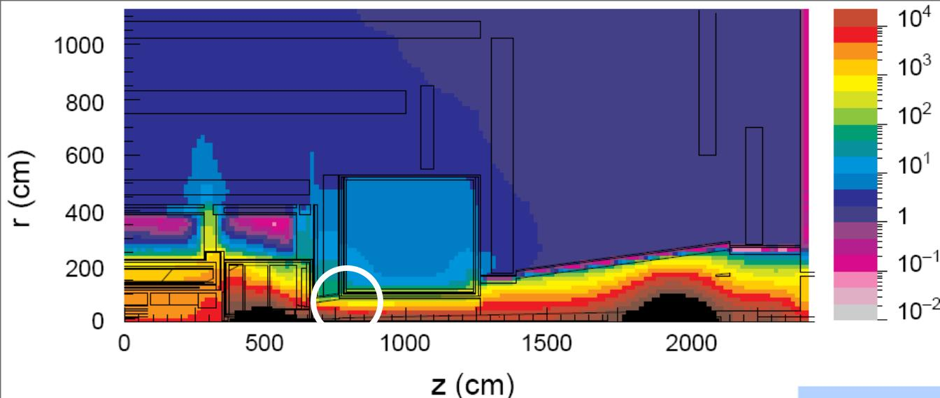
The expected neutron fluence (kHz/cm<sup>2</sup>) in the ATLAS Hall (ATLAS muon TDR, 1997)
