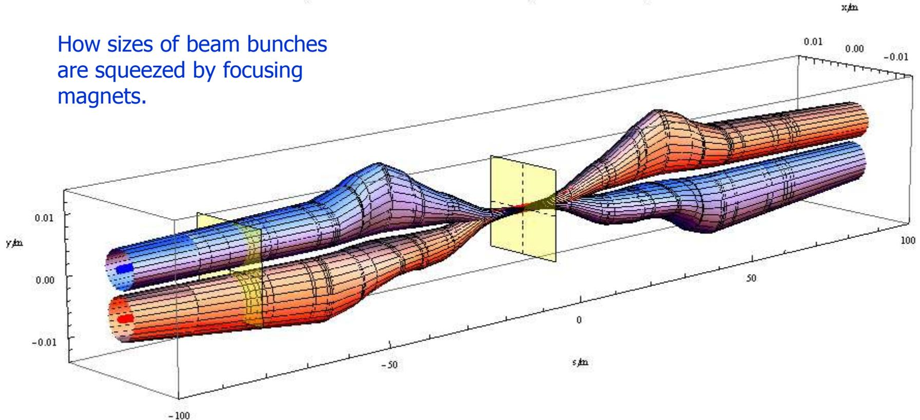
Zero crossing angle at IP (external crossing angle
