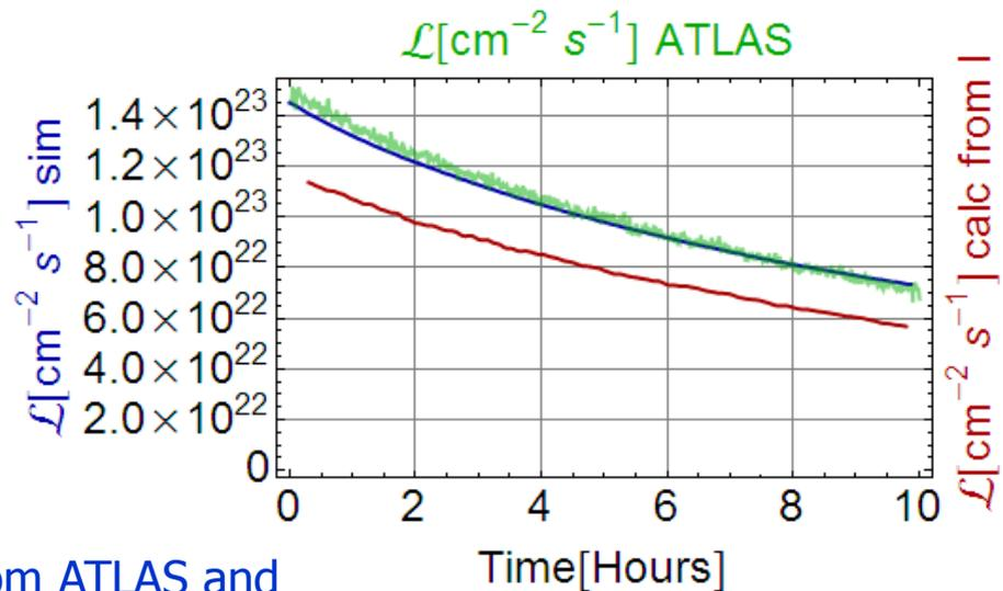
Good fill: after detailed analysis of data from ATLAS and machine instrumentation, there is good agreement with simulation model (non-gaussian IBS, emittance growth, debunching from RF bucket, luminosity burn-off, etc.).
