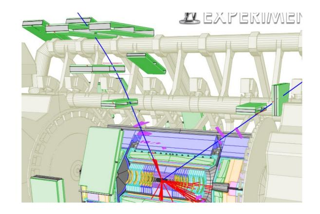
Muon spectrometer particle identification pt measurement
