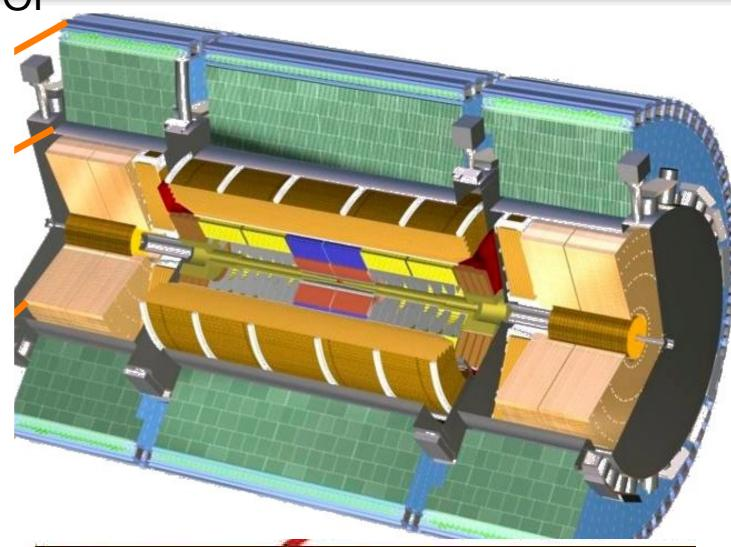
EM calorimeter: Pb-LAr Accordion  $e/\gamma$  trigger, ID and measurement E-resolution:  $\sigma/E \sim 10\%/\sqrt{E}$
