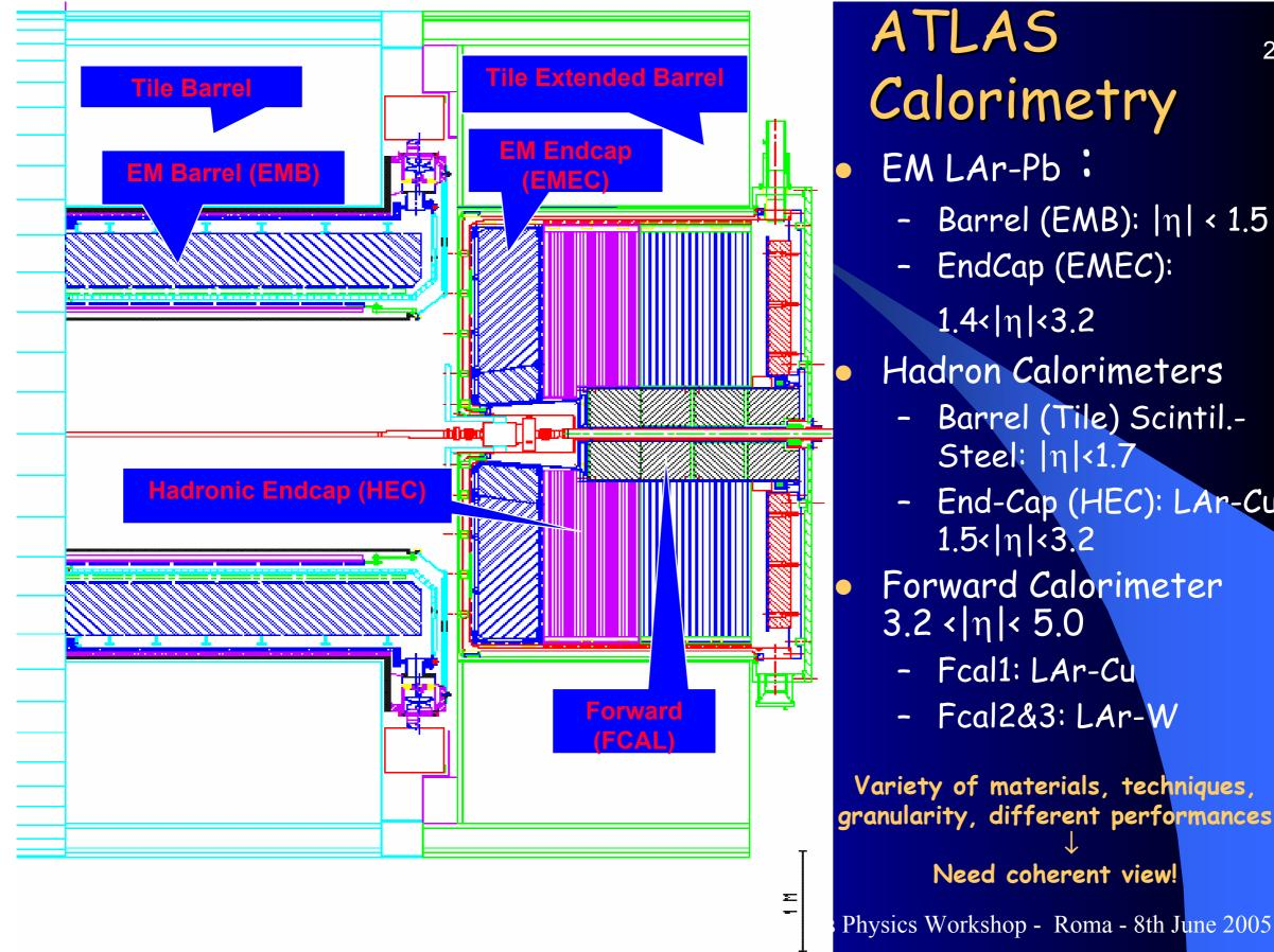
Calorimetry EM LAr-Pb - Barrel (EMB): |η| < 1.5 - EndCap (EMEC): **1.4**<|η|<3.2 Hadron Calorimeters - Barrel (Tile) Scintil.-Steel: |η|<1.7 - End-Cap (HEC): LAr-Cu 1.5< η < 3.2 Forward Calorimeter **3.2 <**|η|< 5.0 - Fcal1: LAr-Cu - Fcal2&3: LAr-W Variety of materials, techniques,
