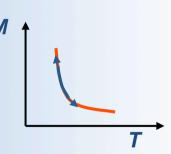
$$\delta M = \frac{\partial M}{\partial T} \delta T = \frac{\partial M}{\partial T} \frac{E_{\gamma}}{C_{\text{tot}}}$$
