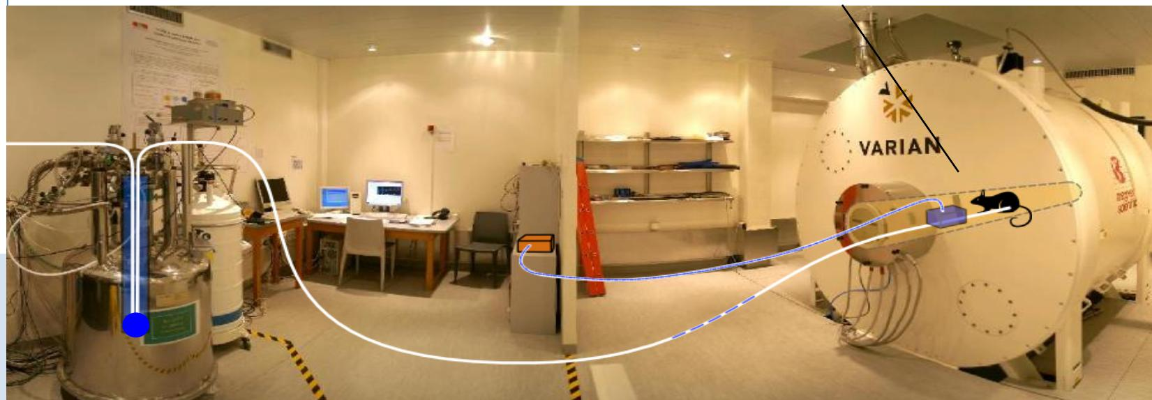
separator/infusion pump located inside the imager
