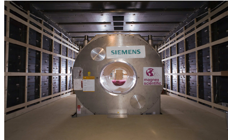
7T Magnet (Siemens/Magnex) (140 000 x earth field)
