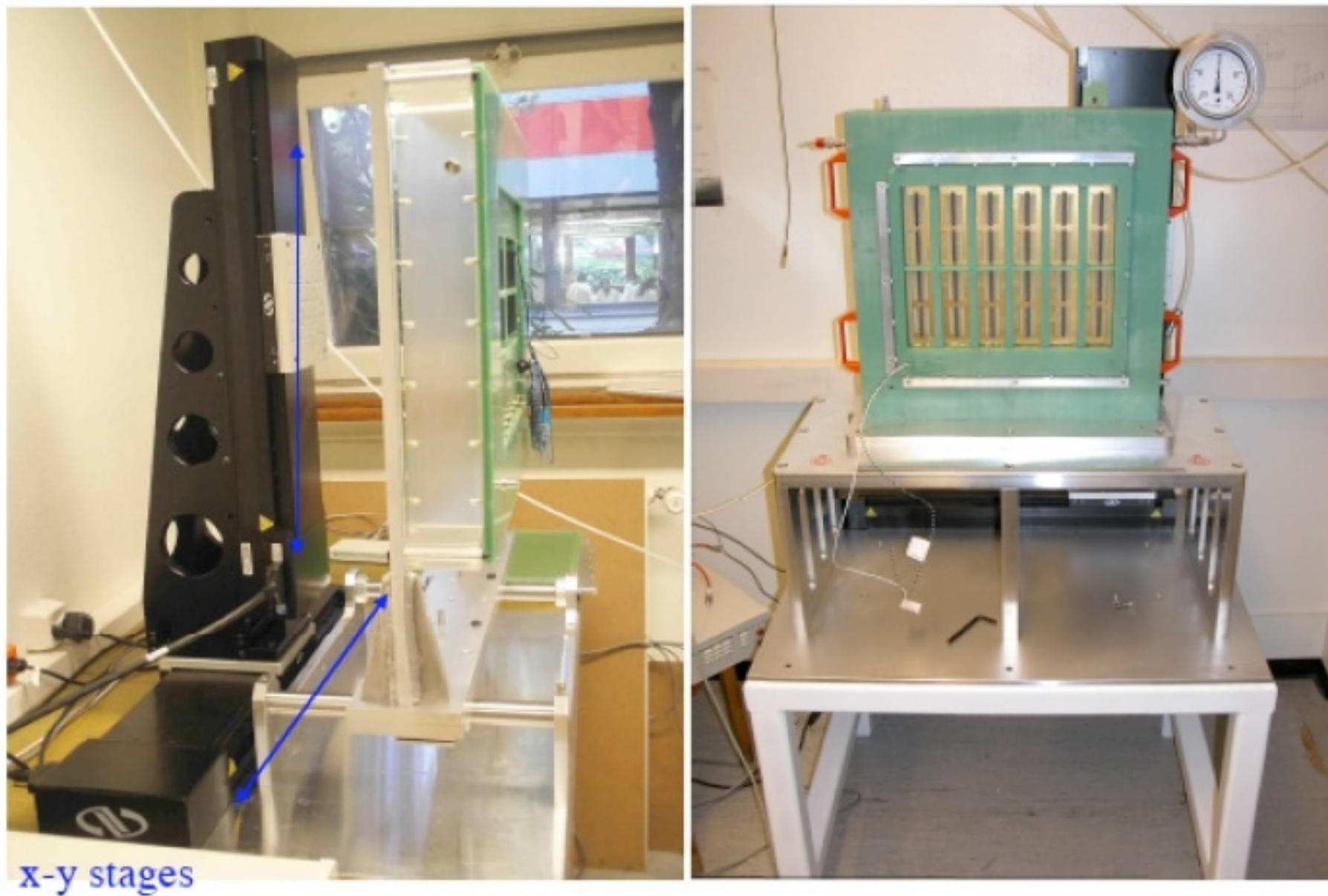
Figure 4.18 : Test bench for final calibration of the MM Modules
