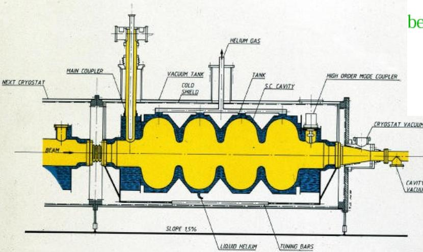
SUPERCONDUCTING CAVITY WITH ITS CRYOSTAT
