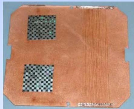
RAD 2: test on small parts (gold wires, heaters, teflon)
