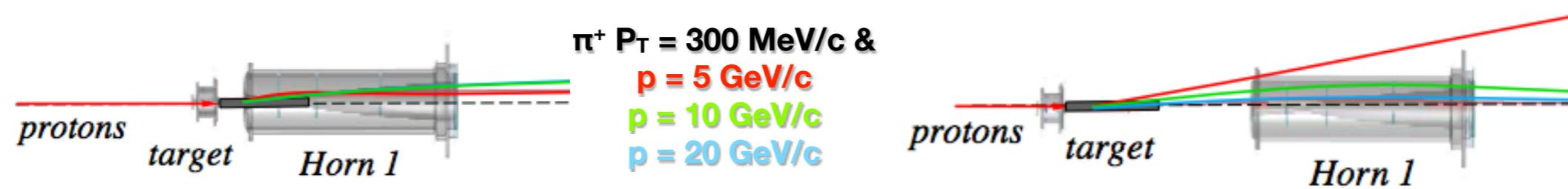
By moving the target and changing the current, we focus different parts of the pion production spectrum.
