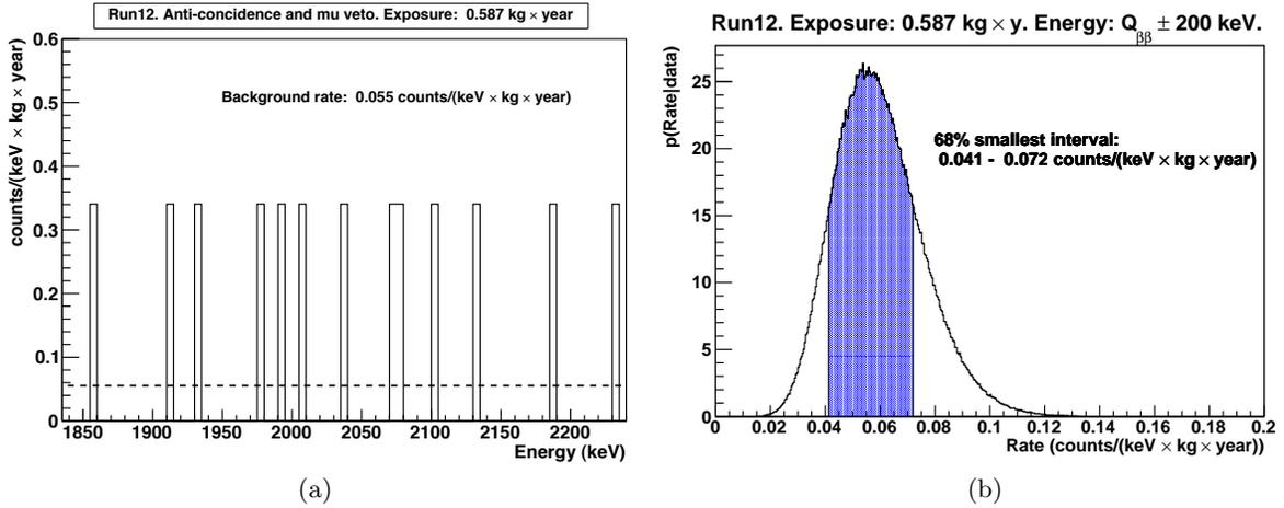
Figure 3: (a) Measured spectrum in a 400-keV-wide window around  $Q_{\beta\beta} = 2039$  keV for run 12. (b) posterior pdf for the background rate given the observed counts in the window. The smallest 68% interval is highlighted.
