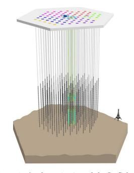
Figure 1: A schematic view of the IceCube detector, with the Eiffel Tower added for scale. There are 86 strings of detector modules deployed within the glacier; where each string connects to the surface, there is a dot. The color of the dot represents the year which that string was deployed.
