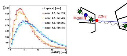
⇒ Resolution of individual crystals (segments) can be determined with a roughly known resolution of one detector.
