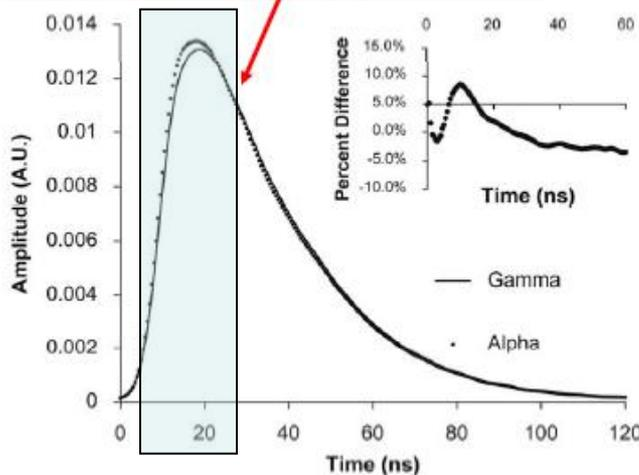
Signal shapes of  $\alpha$ -particles and  $\gamma$ -rays in LaCl3:Ce
