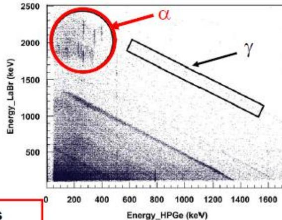
Matrix of coincidence events measured with LaBr3:Ce (y-axis) and HPGe (x-axis) detectors
