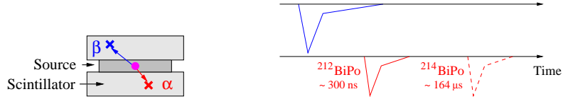
Figure 2: BiPo detection principle with plastic scintillators and time signal seen with PMTs. Dots represent the contamination and crosses represent energy depositions in scintillators (trigger in blue and delayed in red).
