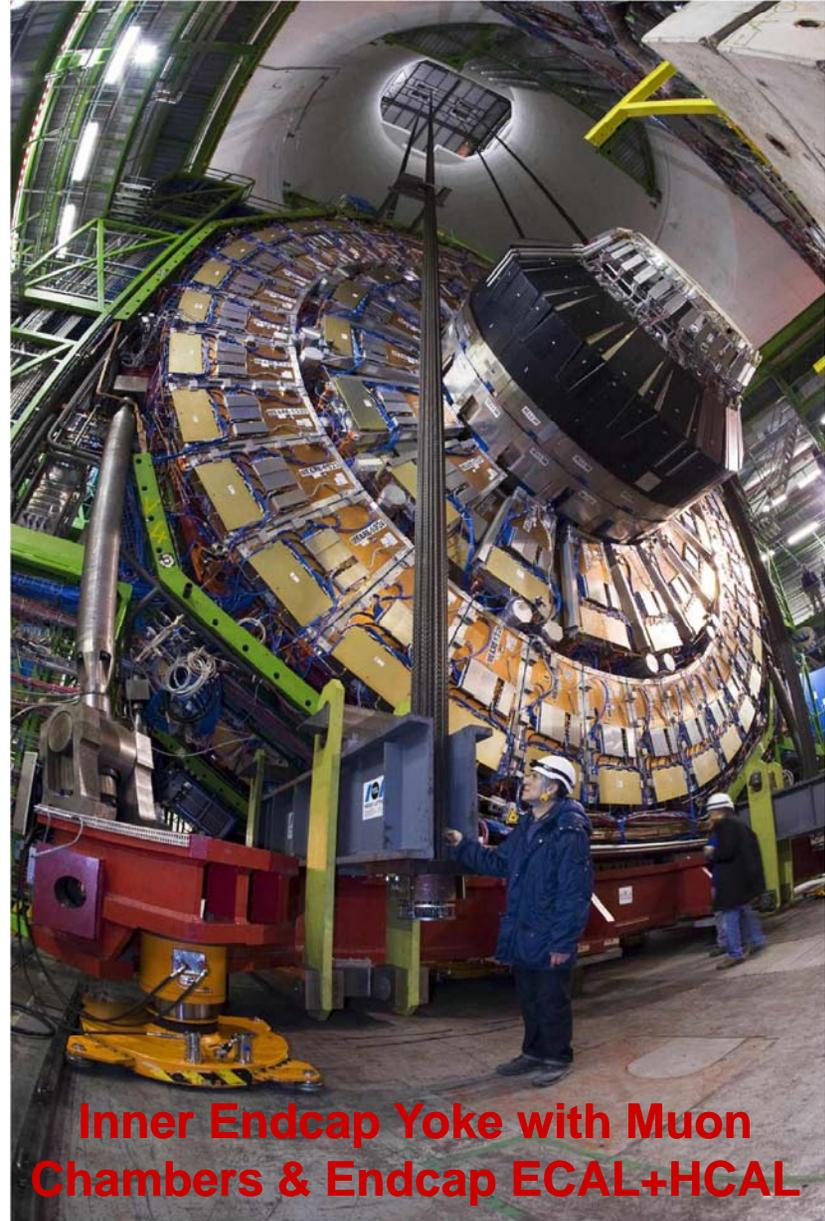
**Inner Endcap Yoke with Muon Chambers & Endcap ECAL+HCAL**
