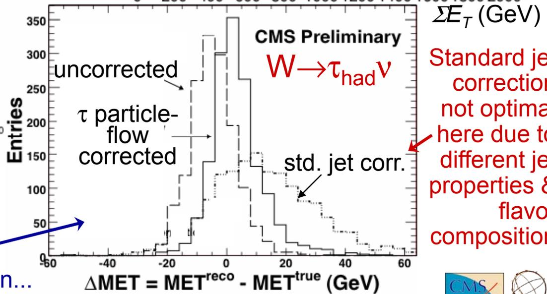
Standard jet correction not optimal here due to different jet properties & flavor composition
