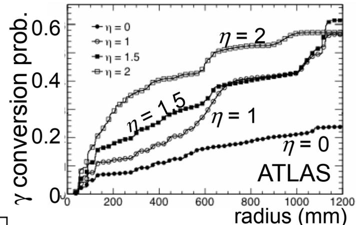
Photon conversion in material before the ECAL !...
