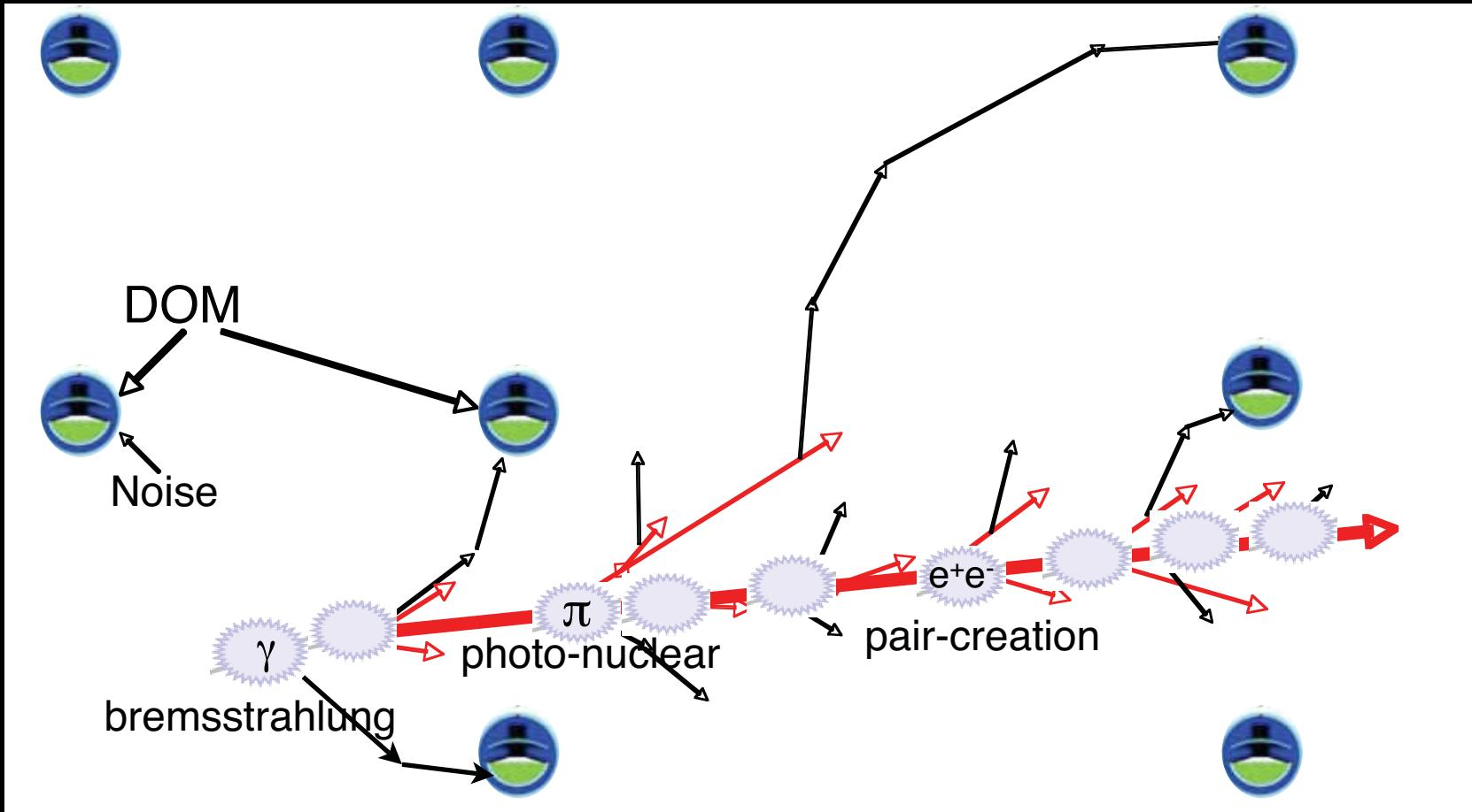
Charged particles emit Cherenkov radiation angle =  $\cos^{-1}(1/n) = 41^\circ$
