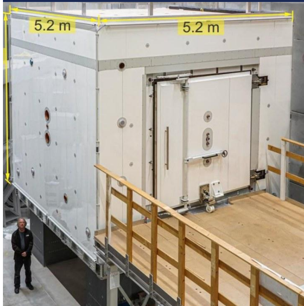
Passive – shielded room
