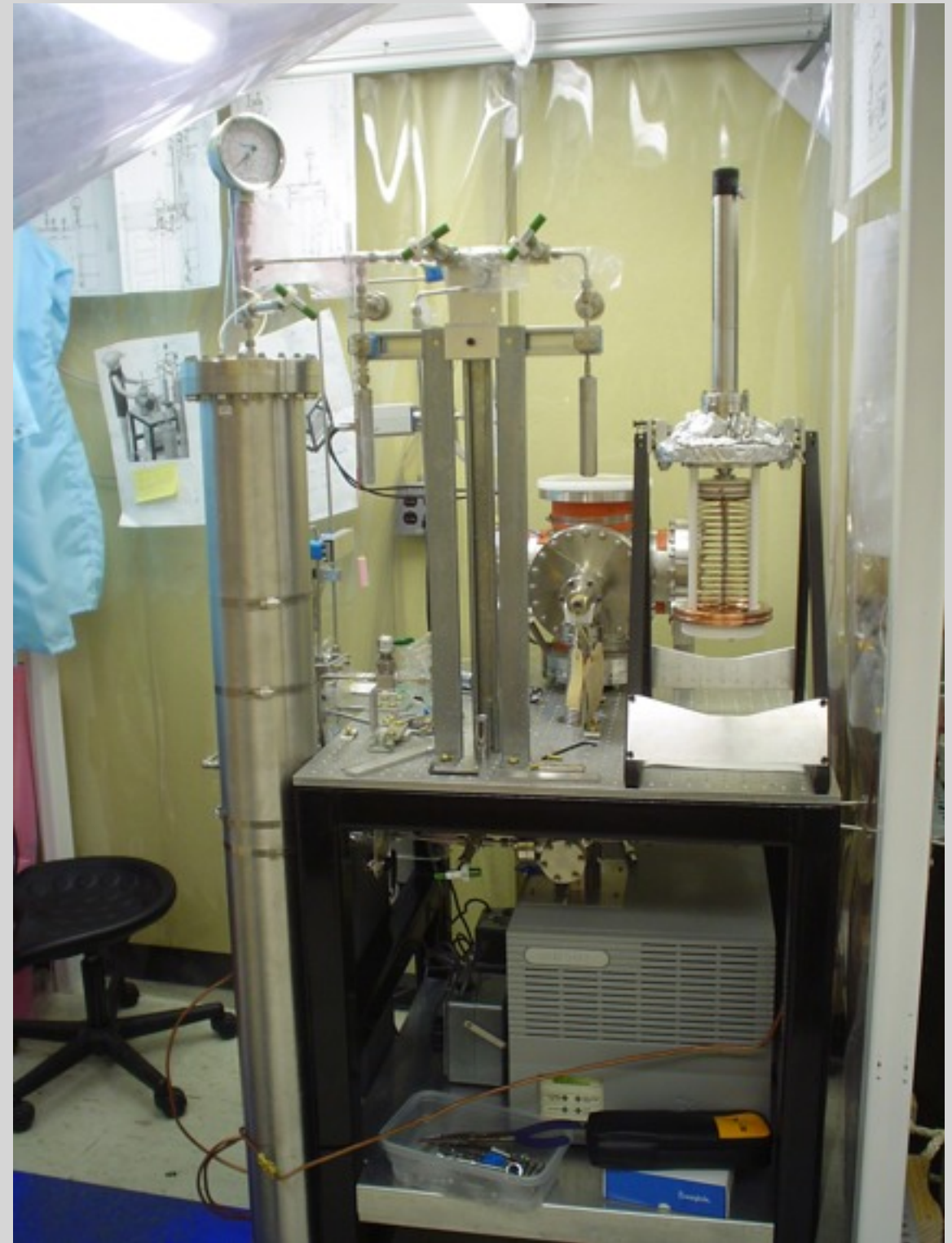
Chamber for studying energy resolution in gaseous Xe at Carleton
