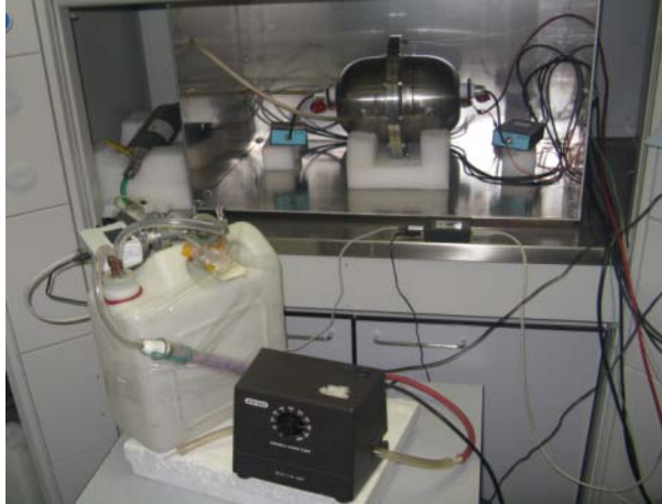
Prague : setup to measure permeability of materials
