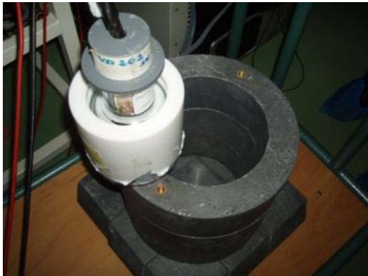
CENBG : setup to measure radon emanation with liquid scintillator
