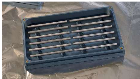
>1200^\circ\text{C} baked Nb rods
